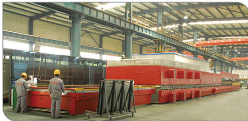
Double Chamber Temper Furnace #1
