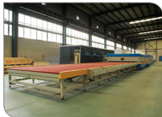
Jumbo Temper Furnace
