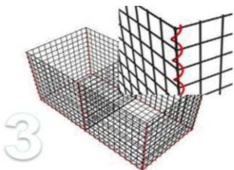
Secure panels by screwing spiral binders through the mesh openings in adjacent panels
