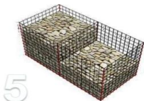
Filed with stones Then close the lid and secure with spiral binders at the diaphragms, ends, front and back
