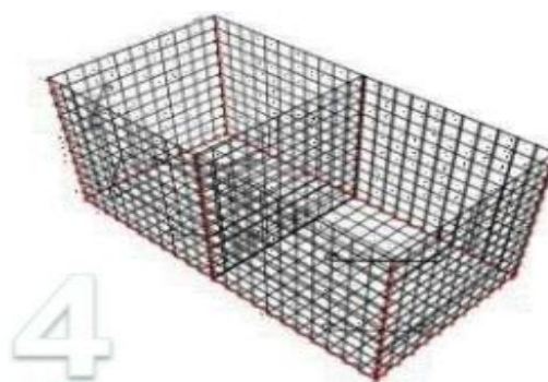
Stiffeners shall be placed across the corners Providing a diagonal bracing, and crimped over the line and cross wires on the front and side faces
